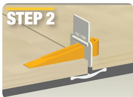
Position the tiles, aligning the sides and pushing them tightly against the clip. Slide a reusable wedge into each clip and tighten until tiles are snug against the bottom of the wedge.
