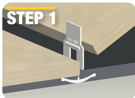
Apply adhesive according to manufacturer's instructions. Vitrex LASH Tile Levelling System is recommended when using at least a 6mm x 6mm trowel depending on tile size to apply the adhesive. Slide two clips under the tile approx. 50mm from each end of the tile.
