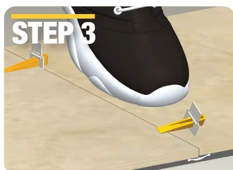
Let the adhesive dry as required by manufacturer's instructions. Simply kick the side of clips in the direction of the grout joints to snap them off or use a non-marking, rubber mallet. Keep reusable wedges for your next project.
